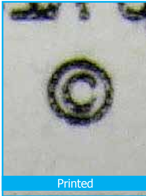
4 pt © Symbol at 70 µm depth (left) and 100 µm depth (right) Traditional method on top Hybrid method on bottom
